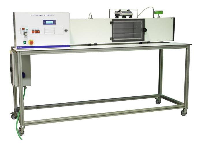
The objective of the IQ 01.5 equipment is to analyze the drying by convection of the element to be studied, modifying the environment in which it is and reflect the data of the changes produced.
